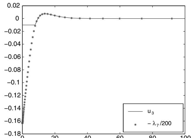
Fig. 12 Control trajectory  $t \rightarrow u_3$  and its switching function.
